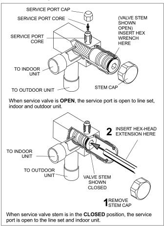
Figure 3. Operating Angle-Type Service Valve
